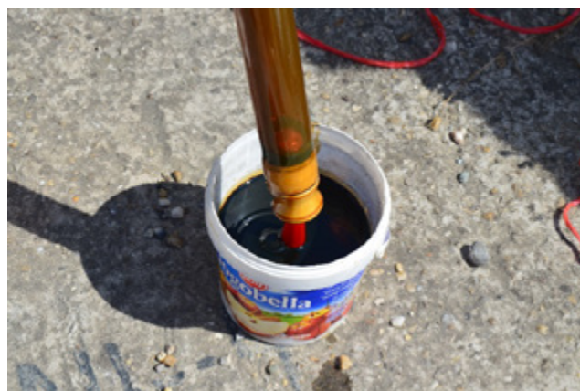
Fig.1 Withdrawn groundwater sample from the VN4-5 borehole polluted by the oil substances (Jantáková, 2017)
