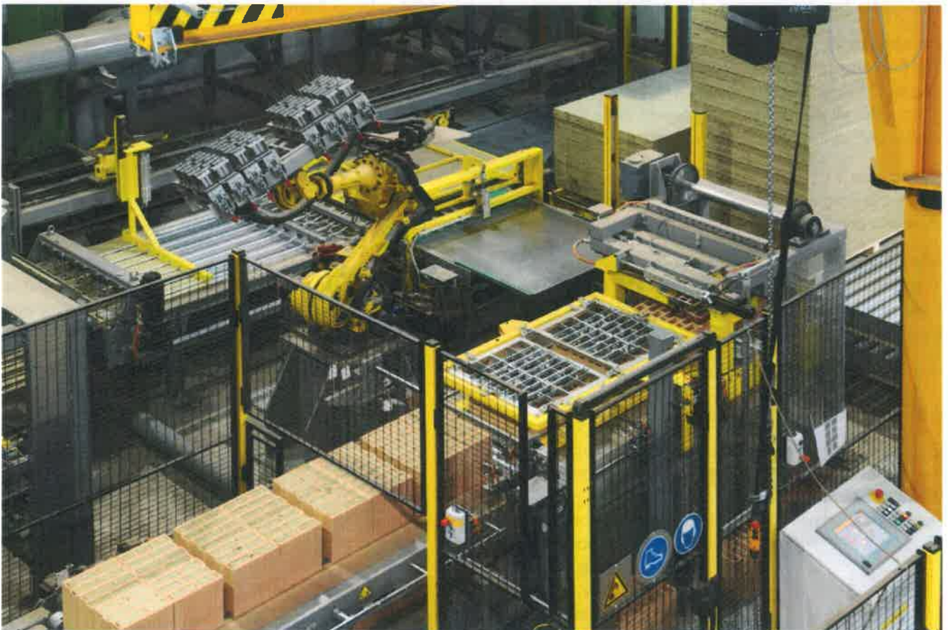
Photo 4 - Inserting thermal insulation into brick blocks
