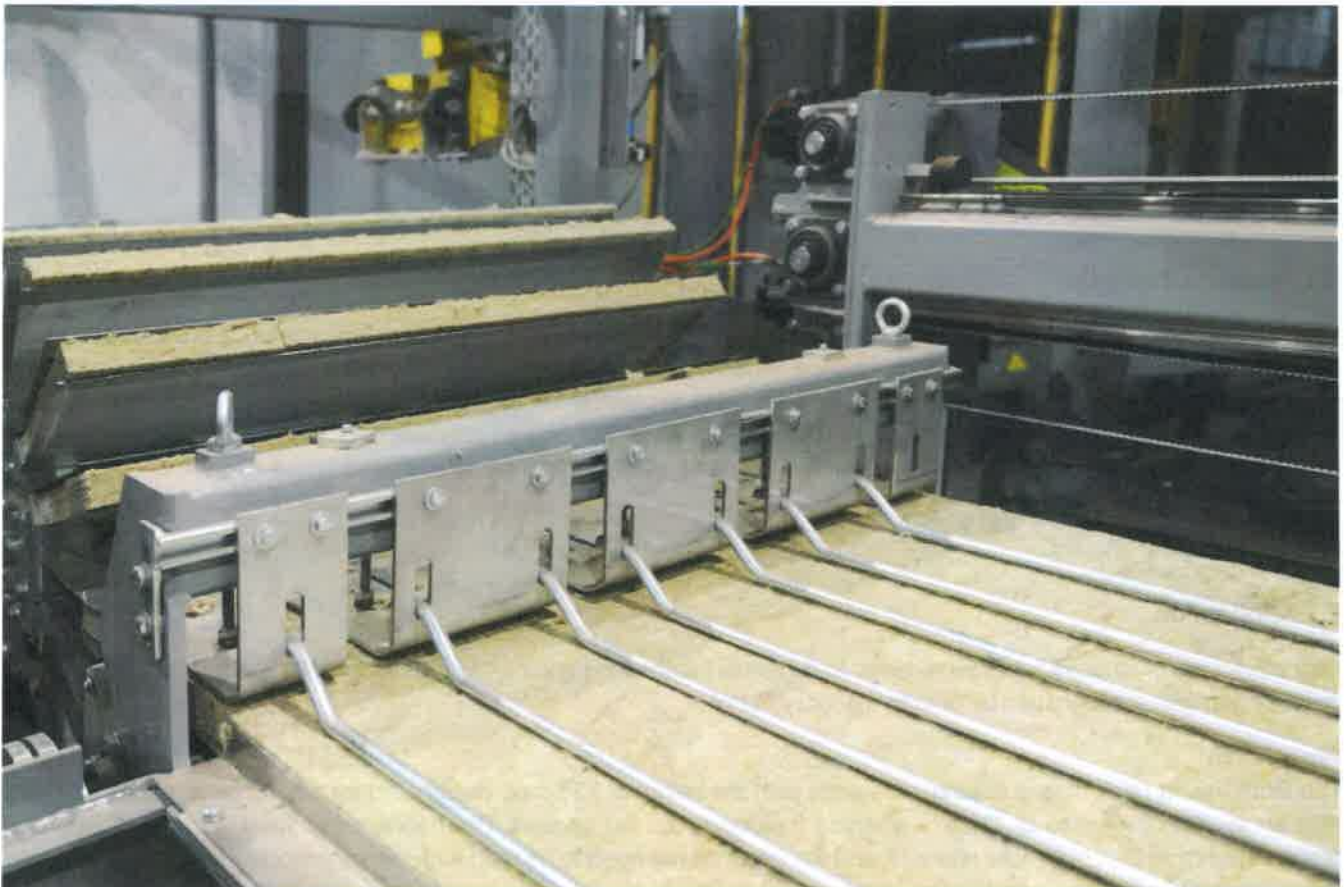
Photo 2 - Thermal insulating pads prepared at carousel
