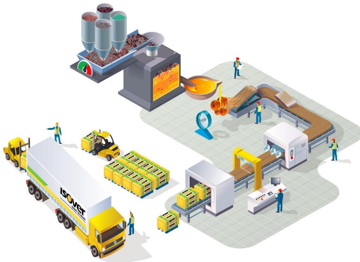
Fig. 3 – Manufacturing process schema
