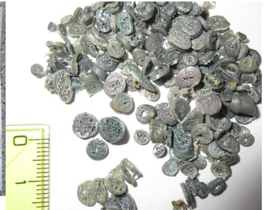
Volatiles make the pellets spongy
